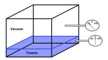
But look what has happened to the pressure differentials. The toluene is still exerting the same pressure as before, as expected, but now, there is a vacuum in the top part of the chamber. How could one possibly have a pressurized chamber at the bottom, and a perfect vacuum at the top?
