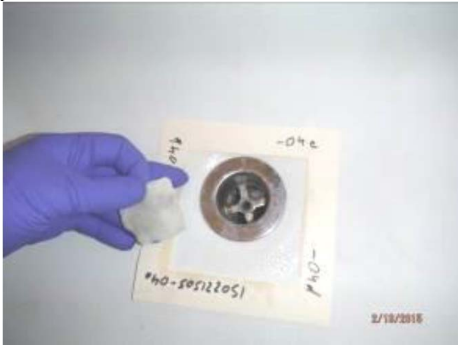
Photograph Documenting Failure to Collect 100cm 2
