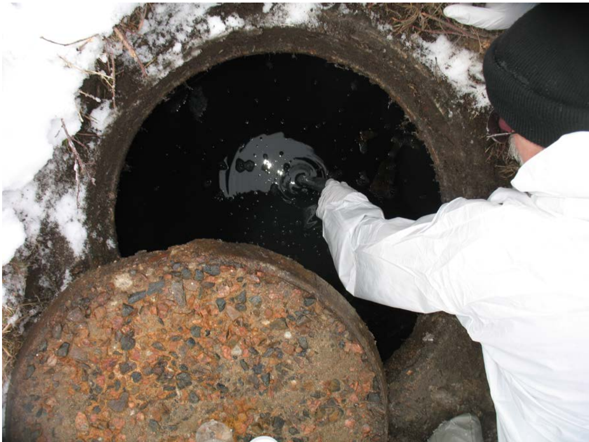
Photograph 2 Coliwasa Stratified Septic Tank Contents
