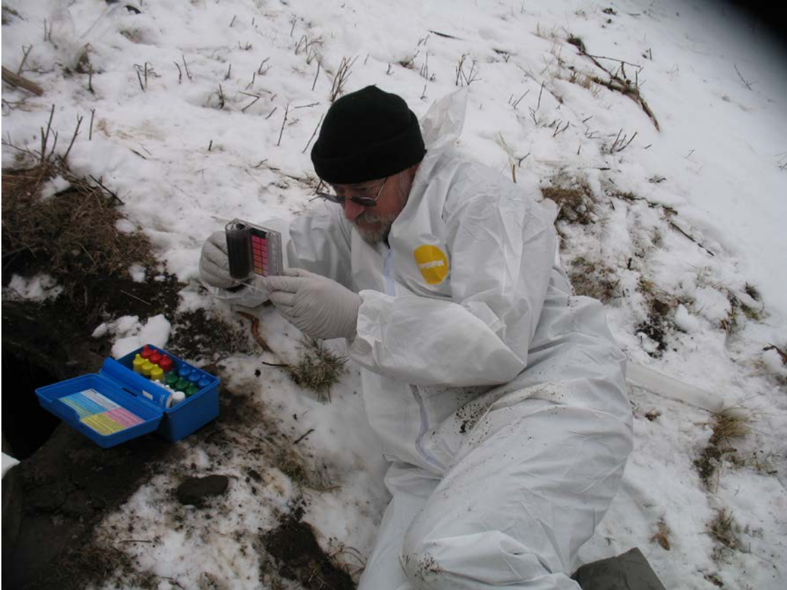
Photograph 3 Wet Chemistry Determinations of Septic Tank Contents
