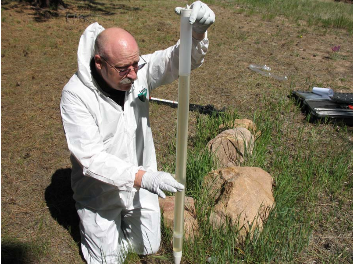
Photograph 2 Coliwasa Stratified Septic Tank Contents
